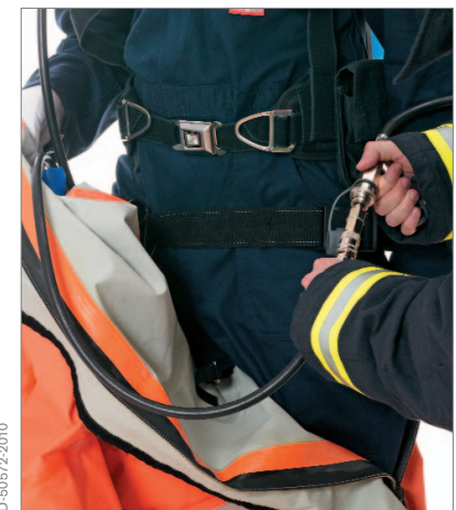
Connection of the air line with the SCBA inside of the suit
